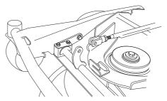
4 Unscrew the bolt holding the unit frame bracket.
